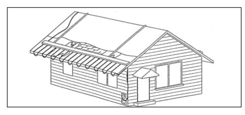
Figure I Cables secured to roof
