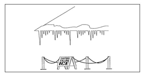
Figure 3 Rope off areas where overhead ice is heavy or slides may occcur.
