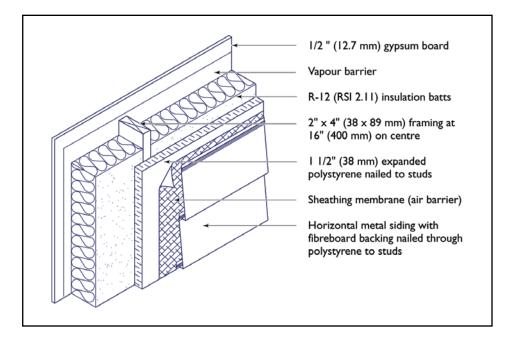
Figure I Effective thermal resistance: R 16.7 (RSI 2.94)
